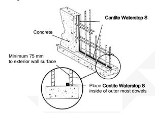
Typical placement of Contite Waterstop S at concrete construction joints
