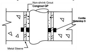
Placement of **Contite Waterstop S** (25x20 mm.) at typical construction joints.
