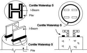
Encircling pile caps metal I-beam and reinforcement Irregular Concrete Surfaces: Follow general instructions above. Press Contite Waterstop S against irregular contours filling cavities and cracks do not leave gaps between water bar and surface. It may prove necessary to install in an irregular direction to avoid major depressions or cracks.
