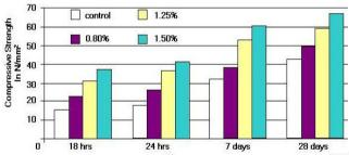
Typical strength development with different dosages of Cormix SP1B cement content 360 kg/m<sup>2</sup>
